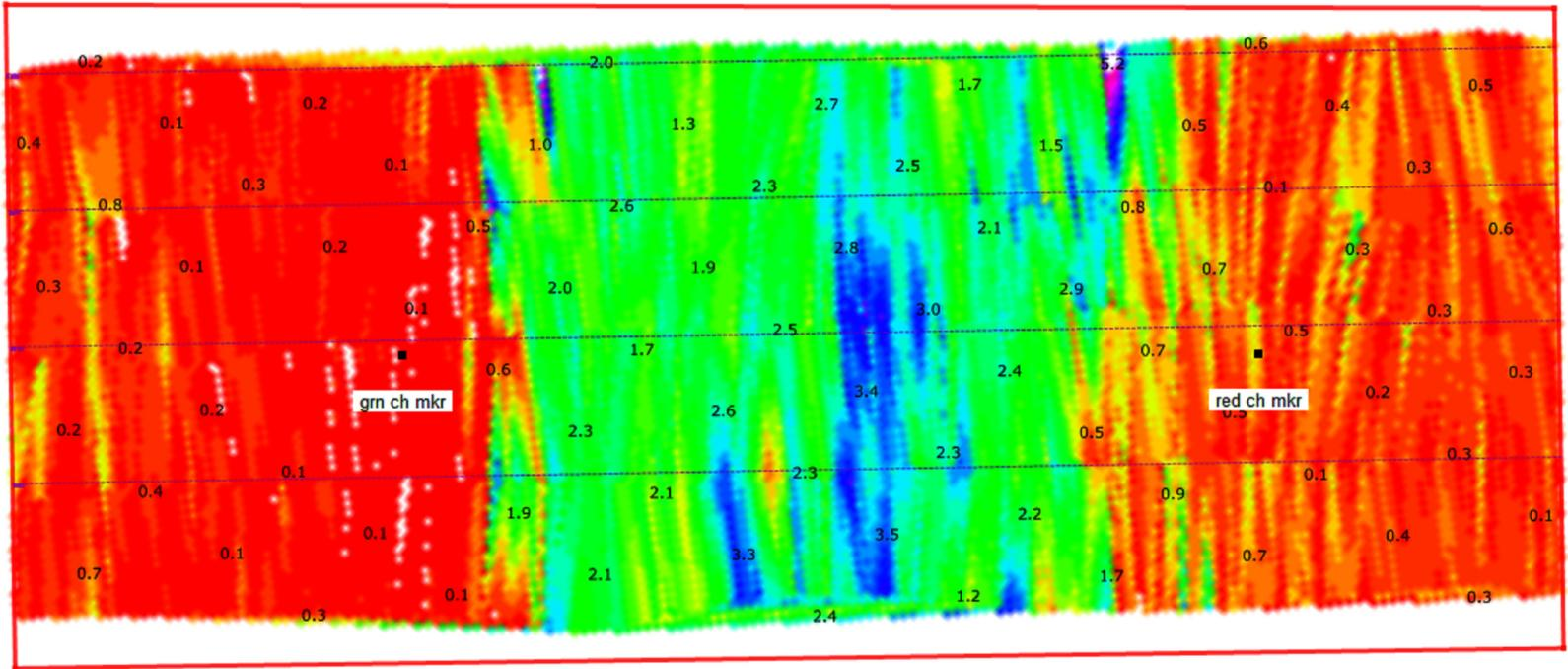
Gulfport Ship Channel LF-HF Mud Layer Thickness (0.25ft)
